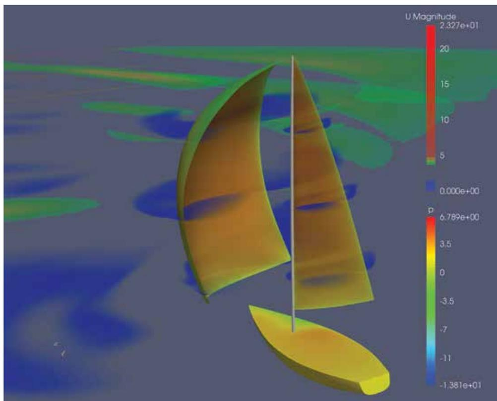
same, only the wing is vertical. Flow over the sail is generated by apparent wind, which is a combination of the true wind and the airflow created by forward movement of the boat.
